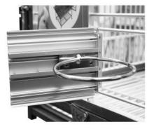
Place the cup ring inside the feeder door track as shown.
