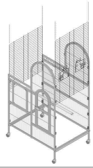
With help holding panels upright, slide the **left and right side panels** down through the channels. ∠
